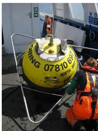
Recovered DWR during inspection and service
